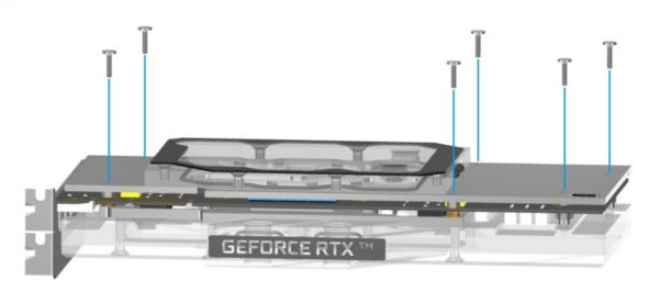
Put the active backplate on and screw it together with the 6 M2x11 screws as shown.
