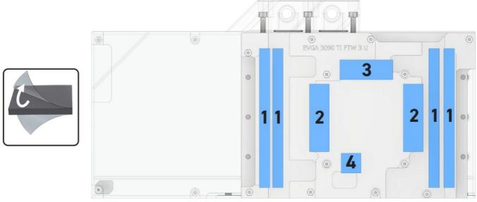
Clean the contact surfaces on the bottom side of the cooler with alcohol or similar. The surface must be free of contaminants.
