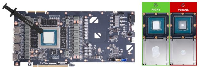
With the help of a plastic strip or similar spread a thin layer of thermal paste on the GPU. The layer should be less than a millimeter thick, otherwise the surrounding components may be contaminated.
