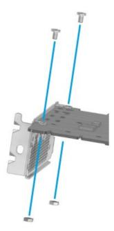
Attach the slot cover as shown using the 2 M3x5 screws and M3 nuts.
