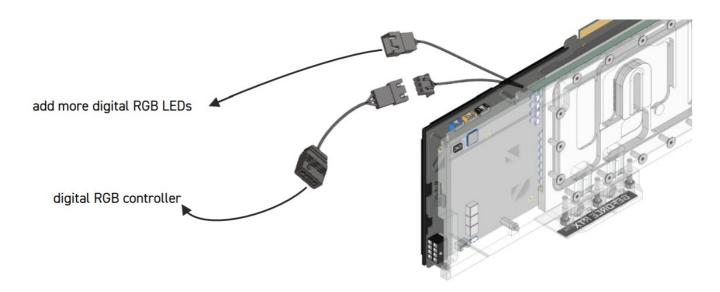
To control the digital – RGB lighting, connect the included adapter to the 3 – pin female connector and plug it to a digital – RGB controller (e.g. Alphacool Aurora Eiscontrol, Art.: 15360, not included). You can connect additional digital RGB LEDs to the remaining 3 – pin male connector.
