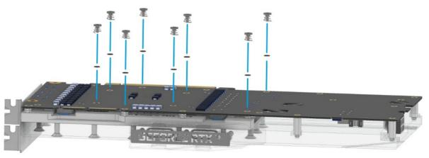
Place the graphics card on the prepared cooler. Fasten the card as shown with the 8 M2x5 screws with M2 washers. Hand-tighten the screws crosswise, one turn at a time.
