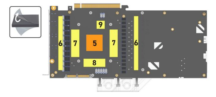
Remove the protective foils from the thermal pads and place the pads on the PCB as shown.
