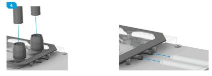
Close the 3mm barbed fittings with the enclosed cap. Screw in the G1/4 screw plugs with the enclosed tool.
