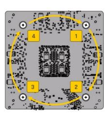
Place thermal pads on PCB backside
