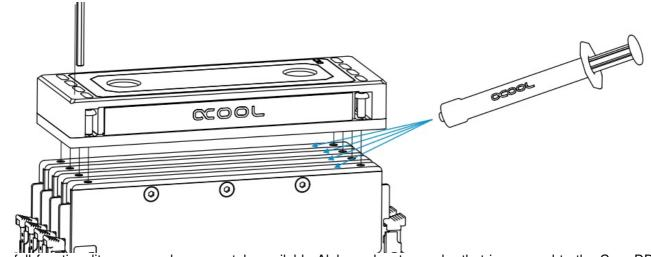
For full functionality, you need a separately available Alphacool water cooler that is screwed to the Core DDR5 modules. The corresponding manual is enclosed with the coolers.
