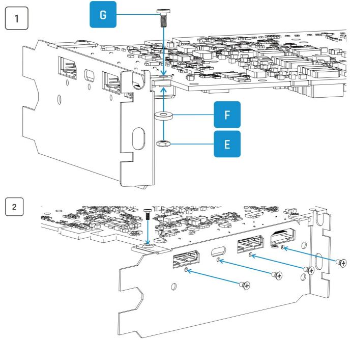
Use the screws supplied in the accessories (1) and the original screws of the graphics card (2).
