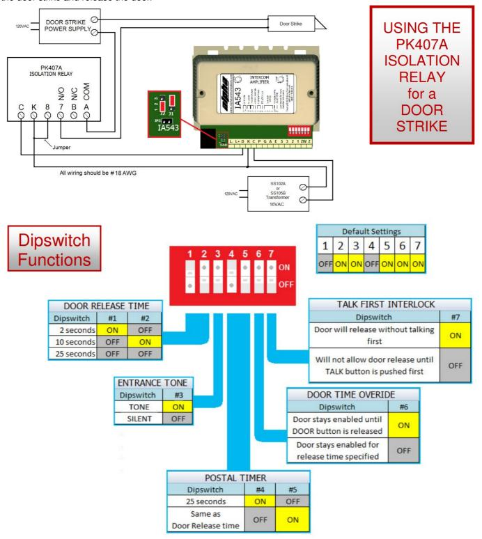
Dipswitches #1 & #2 set the length of door release time for approx. 2, 10, or 25 seconds (See chart above). Dipswitch #3 will provide a tone at the entrance panel when the call button is pressed.
