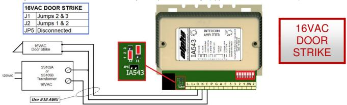
Set jumpers as shown in the chart below. This example shows the wiring for a Multi-Tap Transformer (8/16/24 VAC) to supply 24VAC to a door strike when the inside station DOOR Button is pressed, while also supplying 16VAC for system power. Pay special attention to the transformer wiring and terminal markings. The length of activation time is determined by the dipswitch settings (approx. 2, 10, or 25 seconds).
