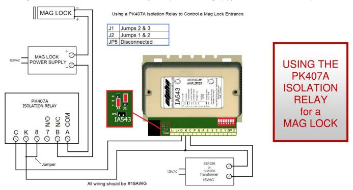
To use the PK407A as an isolation relay for a door strike with a separate power supply, the wiring and jumper settings are the same as above, except the wire going to the B terminal (Normally Closed) would go to the A terminal (Normally Open) instead. This way power from the IA543 would close the connection to apply power to the door strike and release the door.
