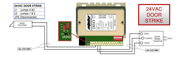
Set jumpers as shown in the chart below. This configuration supplies continuous 24VDC to a magnetic lock through the L+ & L- terminals which is shut off when the inside station DOOR Button is pressed allowing the door to be opened. Insure that proper polarity is observed.
