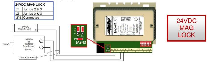
Set jumpers as shown in the chart below. This configuration is used when a magnetic door lock has its own dedicated power supply. The PK407A only provides a dry contact which in this Normally Closed mode, allows voltage to flow to a magnetic lock through the B & A terminals. When the inside station DOOR Button is pressed, the relay opens the circuit, disconnecting the power and releases the door. Insure that proper polarity between the magnetic lock and its power supply is observed.
