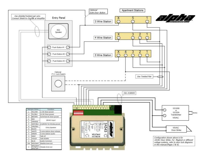
The IA543 amplifier has two serviceable adjustments for Voice Volume and Tone Volume located through two access holes on the front cover. Use a small screwdriver and do not use excessive force. Carefully turn clockwise to increase the volume. High volume setting may result in feedback oscillation.
