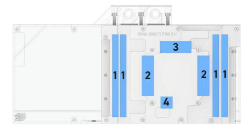
Clean the contact surfaces on the bottom side of the cooler with alcohol or similar. The surface must be free of contaminants.
