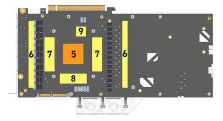
Remove the protective foils from the thermal pads and place the pads on the PCB as shown. **Mounting the backplate**
