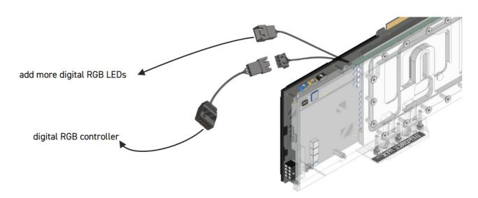
To control the digital – RGB lighting, connect the included adapter to the 3 – pin female connector and plug it to a digital – RGB controller (e.g.
