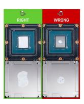
With the help of a plastic strip or similar spread a thin layer of thermal paste on the GPU. The layer should be less than a millimeter thick, otherwise the surrounding components may be contaminated.
