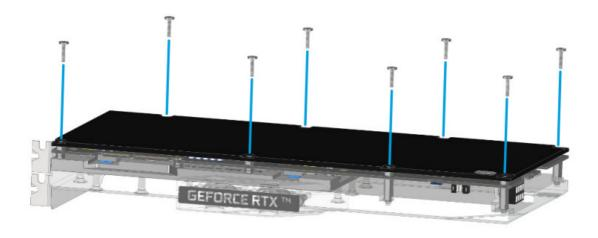
Put the backplate on and screw it together with the 8 M2x11 screws as shown.
