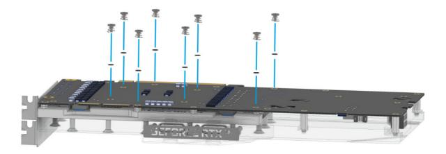
Place the graphics card on the prepared cooler. Fasten the card as shown with the 8 M2x5 screws with M2 washers. Hand-tighten the screws crosswise, one turn at a time.
