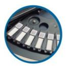
Cartridges are loaded from the center pushing outward until a clicking sound is heard beginning at Position 1.
