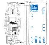
Then fix the panel to the mounting frame using the snaps.
