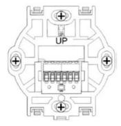
The cable connecting the panel to the controller cannot be run together with the building's electrical wiring. The cable should also not run close to equipment emitting strong electromagnetic field. Drill holes in the wall and, using screws, fix the mounting frame at the desired place on the wall, keeping it in the correct position (UP).
