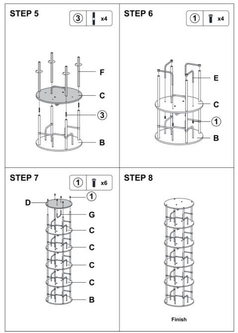
Repeat steps 4, 5 and 6 to install the remaining 3 panel C, and finally install the top panel D
