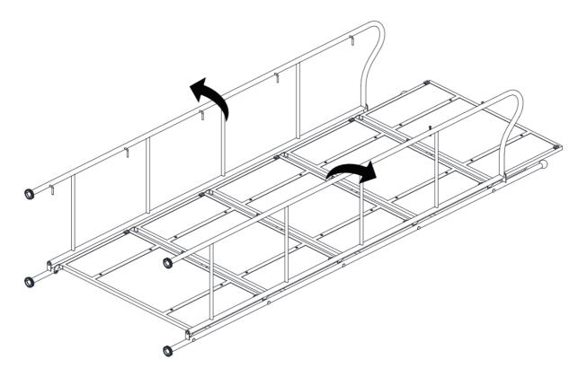
Assemble starting with the shelf 5 from the bottom, unfold and clamp the shelf to the bracket.
