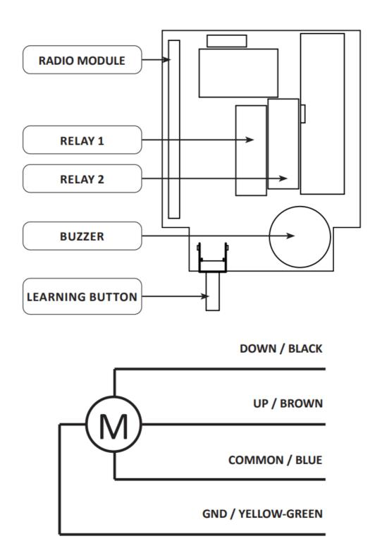
**Warning:** the functions up/down depend on the orientation of the motor. If at one up control corresponds a descent, it will be necessary to invert the brown cable (up) and the black cable (down).
