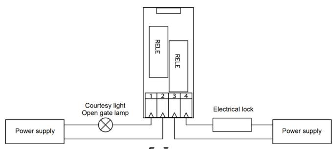
The contact for electrical lock is enabled with the parameter in the advanced menu Maximum load 230 Vac 5A, 30 Vdc 5A max.
