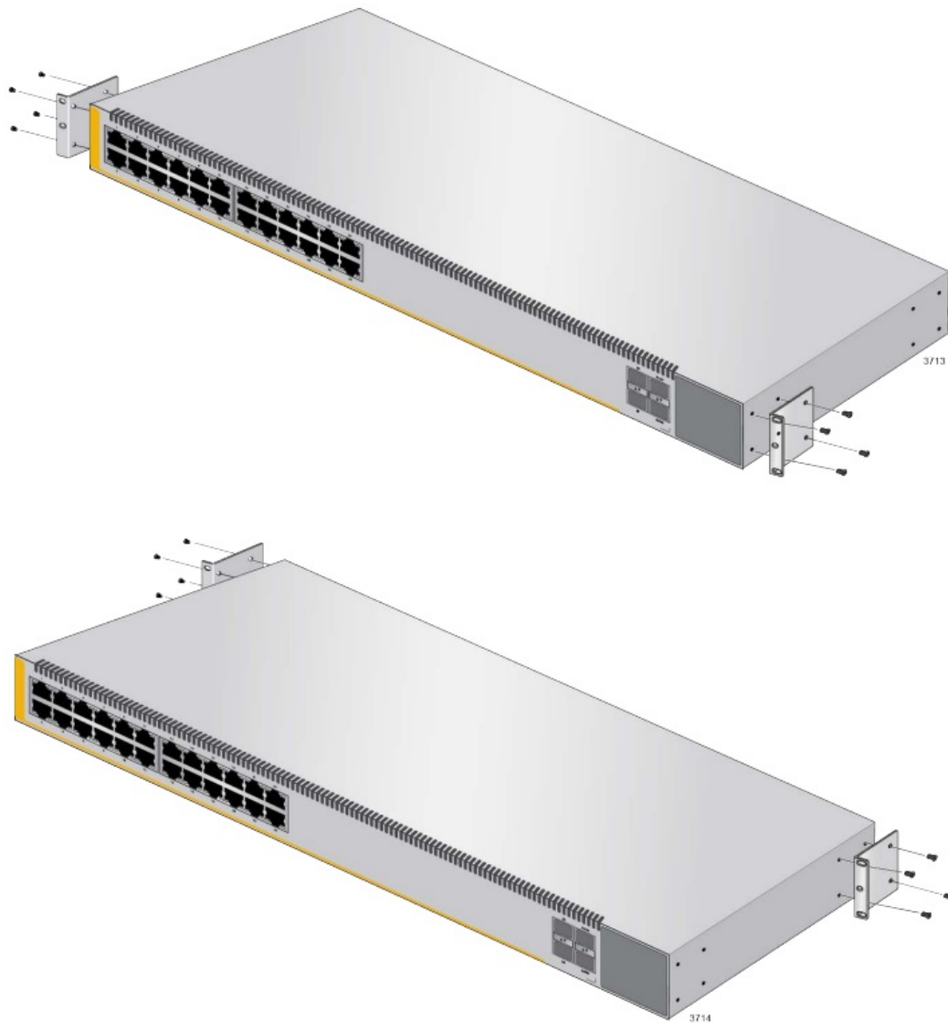
Figure 40. Attaching the Equipment Rack Brackets
