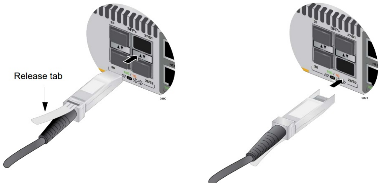
Figure 79. Installing AT-SP10TW Cables
