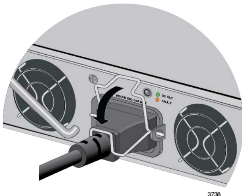
Figure 59. Lowering the Power Cord Retaining Clip
