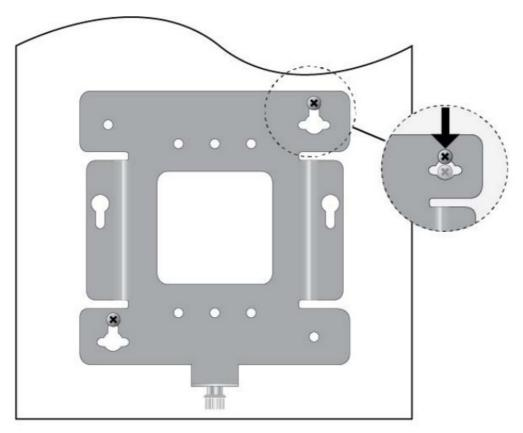
6. Tighten the screws snugly onto the bracket.
