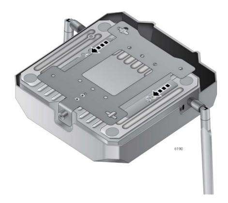
3. Slide the mounting bracket forward and remove it from the access point.
