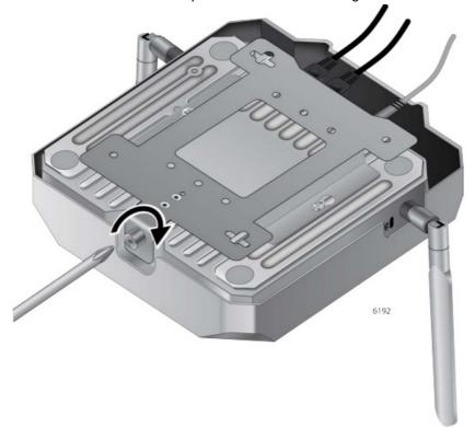
4. Place the Ethernet cable(s) and power cable (if any) along the cable guides inside of the top cover in the cable hiding space.
