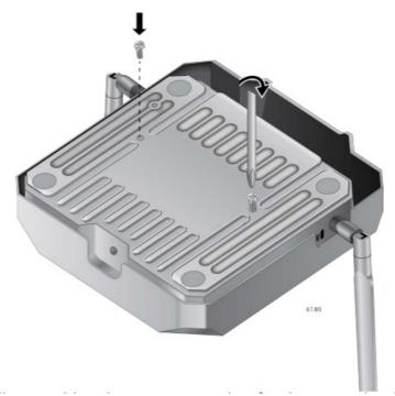
The screw collar provides the proper spacing for the mounting bracket beneath the screw head.
