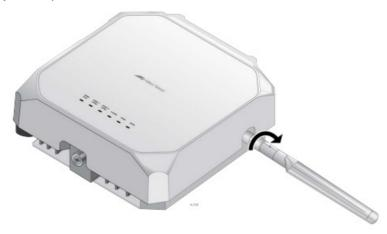
5. Repeat the procedure to attach the other antenna to the other side of the access point.
