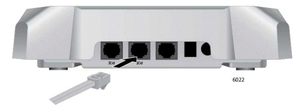
2. Connect the other end of the Ethernet cable to a network device, such as a switch or router.
