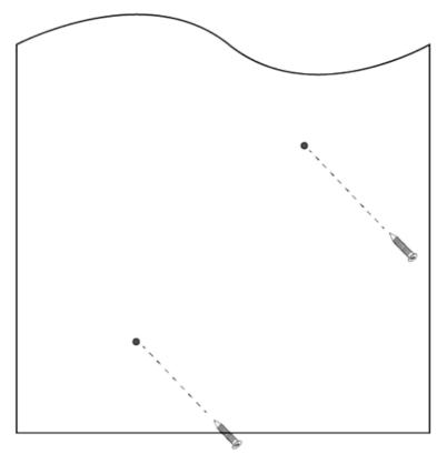
5. Install the openings of the bracket key-hole slots to the two screw heads and slide the bracket into the narrow end of the key-hole slot openings.
