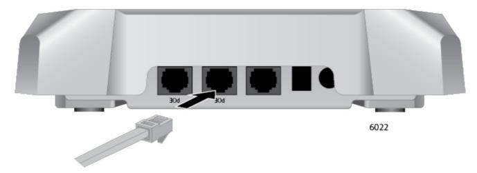
2. Connect the other end of the Ethernet cable to a network device, such as a switch or router.
