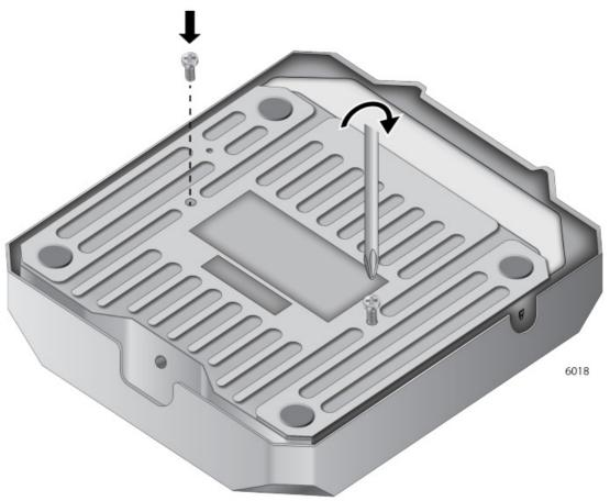
2. Install the two screws (provided) fully into the bottom panel of the access point. The screw collar provides the proper spacing for the mounting bracket beneath the screw head.
