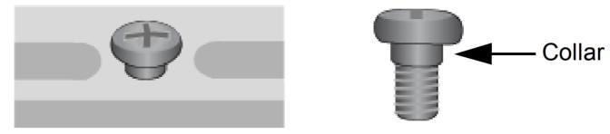
3. Make sure that the mounting bracket fits to the access point by sliding the bracket beneath the screws.
