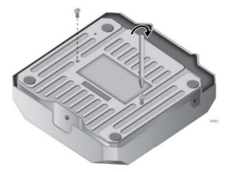
The screw collar provides the proper spacing for the mounting bracket beneath the screw head.
