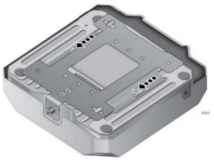
4. Slide the mounting bracket forward and remove it from the access point.
