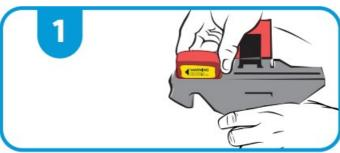
Roll RapID Evo Tags towards you firmly. Bias the pins outwards to avoid jamming.
