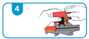
Depress the clamp (A) firmly. Slide tags out until location lugs are between first and second tags.
