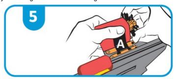
Pull trigger to move tag into the Load position.
