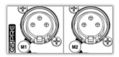
Avoid 'hot plugging' when connecting any equipment and make sure AUX MASTER and MAIN MIX controls are turned down before 48V is switched on as this as may cause loud thumps and bangs!
