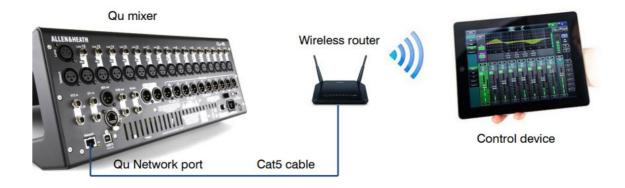
The Qu mixer firmware and app versions must be compatible. For example, V1.9 app will not run with V1.8 firmware. To avoid unexpected version mismatch we recommend you turn off 'auto update' on your device. Download the latest Qu mixer firmware from the Allen & Heath web site.
