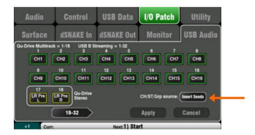
Patch the USB outputs – Use the Setup / I/O Patch / USB Audio screen to patch any of the Qu outputs to the Qu-Drive multitrack and rear panel USB B streaming port. These share the same patch. USB streaming uses all 32 outputs. Qu-Drive recording is fed from the first 18 outputs. Qu-Drive stereo recording is fed from outputs 17-18. Live show multitrack recording typically uses the channel Insert Sends so that live mixing does not affect the recording.
