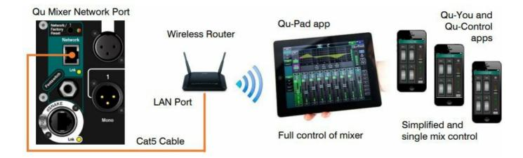
**Wireless router setup** – Connect the router to a PC or Mac using a Cat5 cable. Follow the instructions provided by the router manufacturer to access its setup menus. Once set up, disconnect the router from the computer and then plug it into the Qu mixer Network port using a Cat5 cable.
