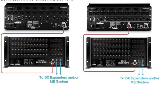
The connection of 2x GX4816s is supported via the use of both the internal SLink port and the optional SLink I/O module.
