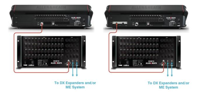
Connection of up to 3x GX4816s is supported via the use of both the internal SLink port and up to 2x gigaACE I/O modules.
