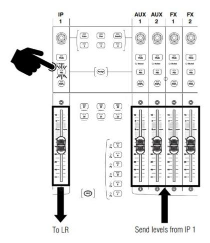
Press an Input Channel strip Mix key (i.e. IP 1) Use this to work with Aux and FX sends. The Input strips remain as Channel Faders.
