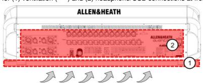
Leave adequate space for (1) ventilation ( ^ ) and (2) audio/power connections at rear of mixer.
