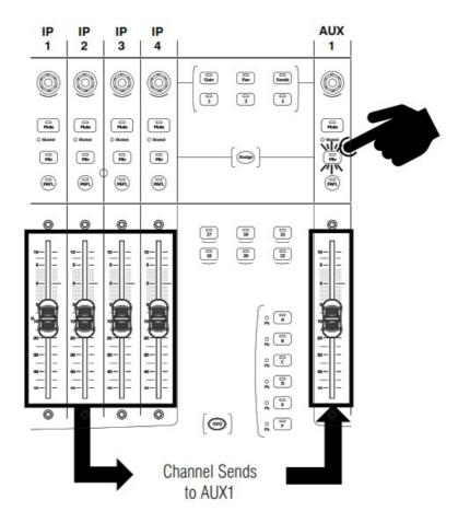
Press a Mix master strip Mix key (i.e. AUX 1) Use this to work with Aux and FX sends. The Input strips present all the send levels to the active Mix. The Master strips present the master mix faders.
