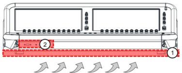
Leave adequate space for (1) ventilation ( ^ ) and (2) headphone/USB connections at front of mixer.
