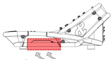
Leave adequate space for ventilation ( \*) at the sides of the mixer in the area indicated.
