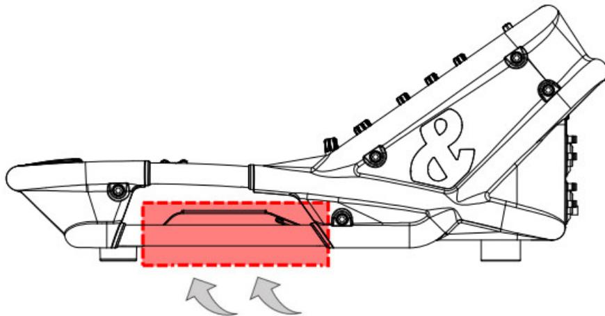
Leave adequate space for (1) ventilation (↗) and (2) USB / headphone connections at front of mixer.
