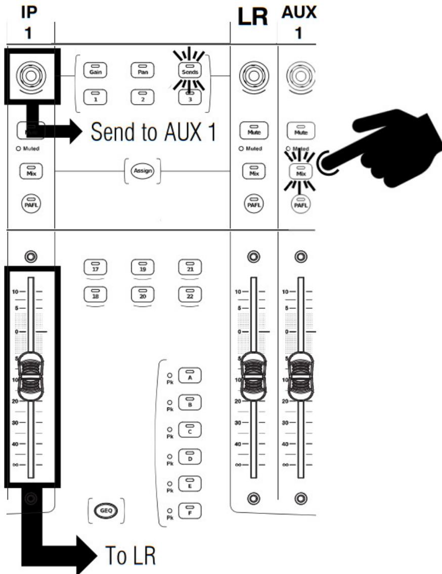
In Sends on Rotaries mode, Strip Rotaries are used to control send levels to the active mix, with the channel faders remaining as level controls to the Main Mix.
