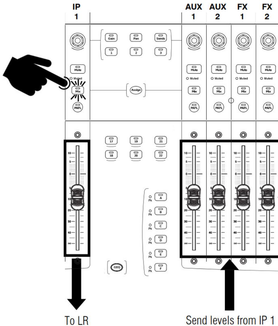
Press an Input Channel strip Mix key (e.g. IP 1)
