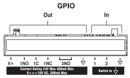
Use the provided 10-pin Phoenix connector with strain relief for optimal cable management.
