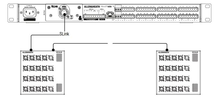
• A DX Hub can be connected to the SLink card for further expansion with up to 8 DX expanders. It also enables a single cable link to the AHM processor in cases where multiple expanders are located on a different floor, area or building.
