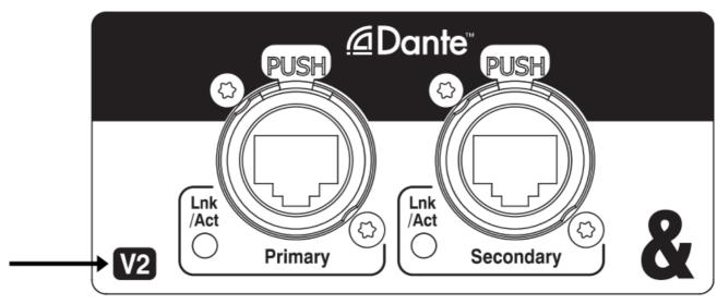
The I/O Port panel is also used to access DIP switch 6 for network reset of the unit to default settings. Reset occurs with switch 6 in the On position at power up. After 10 seconds, turn off the unit and move the switch back to the Off position. Do not alter the position of the other DIP switches.
