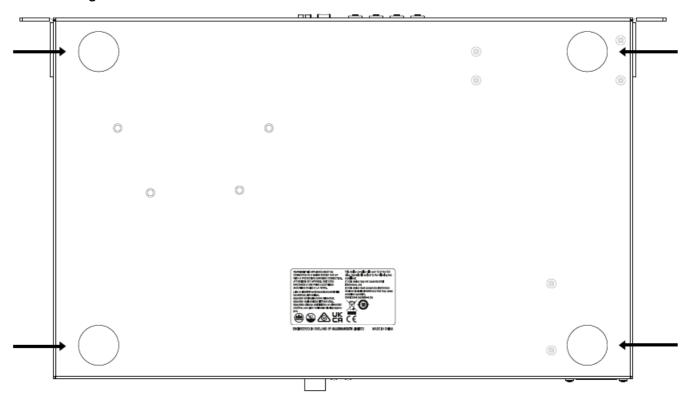
For free standing or shelf operation, apply the adhesive plastic feet to the positions indicated below.
