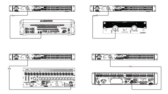
Set the Audio Sync options so that one device is the clock leader (set to 'Internal) and the other device is a dock follower (sync from SLink or I/O Port as appropriate).
