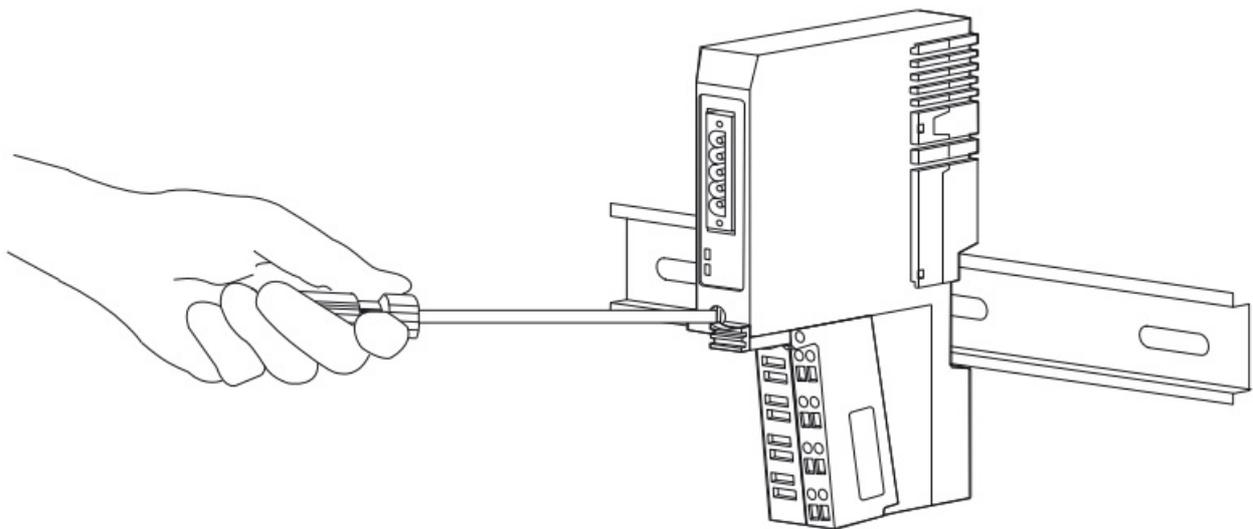
5. Pull the adapter off the DIN rail to remove it from the existing system.
