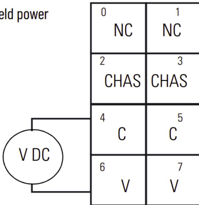
Connect this DC supply to the internal power bus.
