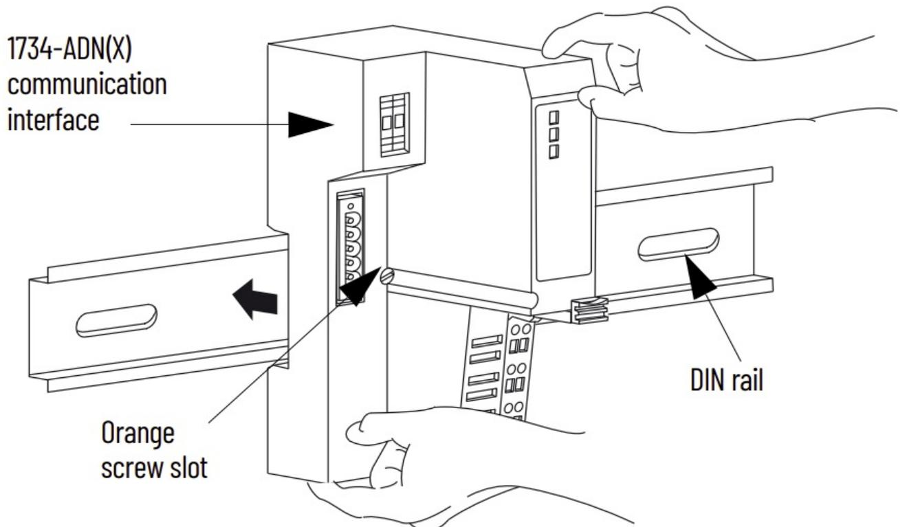
3. Insert the DeviceNet network plug and tighten the holding screws.
