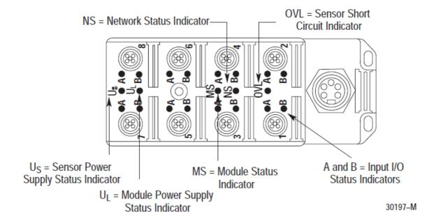
**Note**:This module contains a circuit to protect the DeviceNet power supply from short circuits in an attached sensor or sensor cable. If you connect a sensor while the module is powered, the surge current produced by the sensor can cause the module to fault. This operation is normal.
