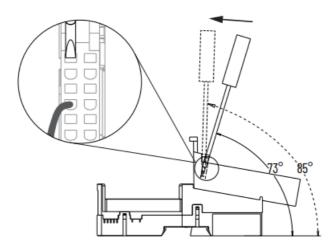
• **WARNING:** For 1734-TOPS and 1734-TOP3S, to latch and unlatch the wire, insert a bladed screwdriver (catalog number 1492-N90 – 3 mm diameter) into the opening at approximately 97° (blade surface is parallel with top surface of the opening) and press in (do not push up or down).
