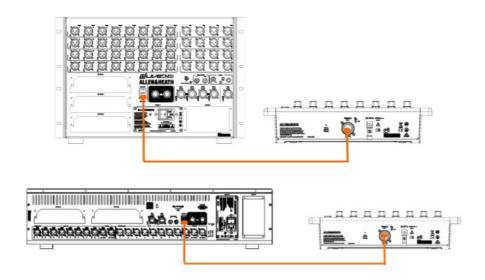
Power up the IP8 by plugging the external PSU into the DC In socket. The port Lnk/Err indicator flashes at a steady rate when the link is established. The unit Name and IP address are displayed on the LCD Displays for easy identification of the unit. After a few seconds the IP8 will display the assignments and functions if any have been set for the unit.
