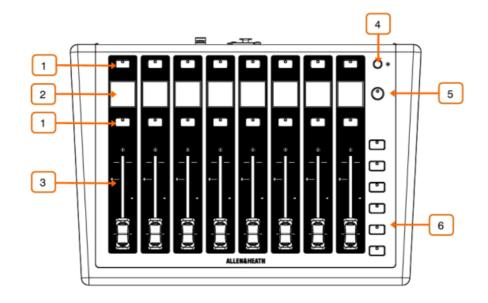
[1] **SoftKeys** – 2 sets of 8x backlit assignable keys. Can be configured individually or as part of a vertical 'Rotary Strip'. Available functions include Send On/Off, PAFL, Mute, Scene Recall, Tap Tempo, Talkback Assign, Custom MIDI. [2] **LCD Displays** – 8x colour displays providing information on the channels and on the function of the SoftKeys.
