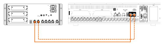
Switch on the Surface. The gigaACE Lnk/Err indicators flash at a steady rate when the link is established. The red error indicator lights if a communication error is detected. Check that the cables are correctly plugged in and are not faulty. It takes around 30s for the Surface to take control and the touchscreen to become responsive.
