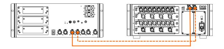
Switch on the DX Expander. The DX port Lnk/Err indicators flash at a steady rate when the link is established. The red error indicator lights if a communication error is detected. Check that the cables are correctly plugged in and are not faulty.
