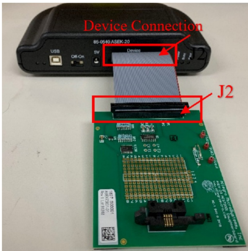
Figure 8: Connection between ASEK-20 and ASEK70311 Daughterboard
