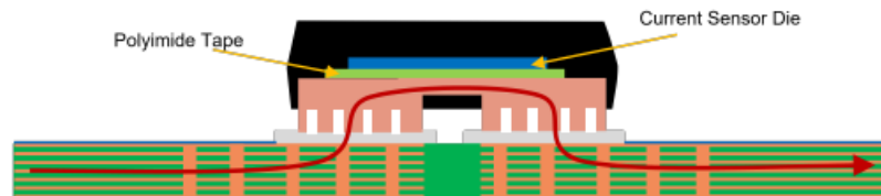
Figure 4: Vias Under Copper Pads Example
