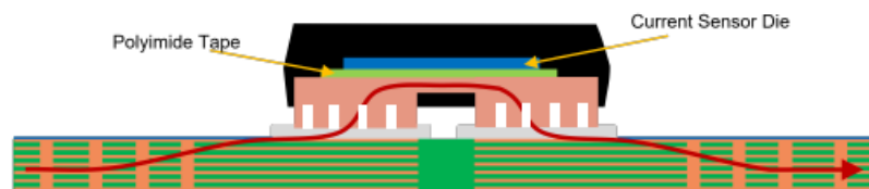
Figure 5: No Vias Under Copper Pads Example
