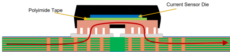
Figure 4: Vias Under Copper Pads (not to scale)
