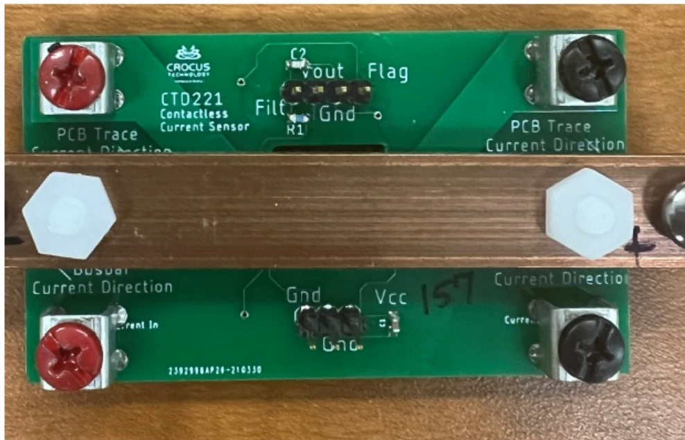
Figure 2: CTD221-BB-1.5 Evaluation Board with Busbar
