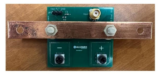
Figure 2: CTD455-BB-06B5 Evaluation Board with Busbar
