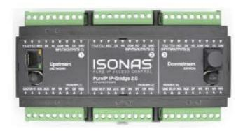
The IP-Bridge 2.0 connects the modern IP-network world and legacy wiegand installations. Simply unplug existing panels and attach wiegand readers directly to the IP-Bridge 2.0.
