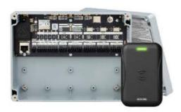
This single opening controller allows perimeter and common area openings to be managed in a single system. **Applications**: Perimeter Exits, Amenity Spaces, Common Areas.
