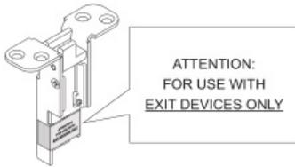
**3b** Connect cable end fitting(s) to latch(es).
