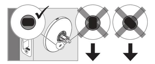
Slot not horizontal? Gently insert pin into slot and rotate to the left until it stops. Confirm the position again.
