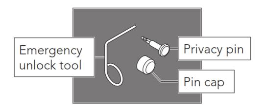
Installing the privacy pin changes the function of the lock from non-locking to locking. AFTER installing interior chassis and trim, but before installing the knob/lever:
