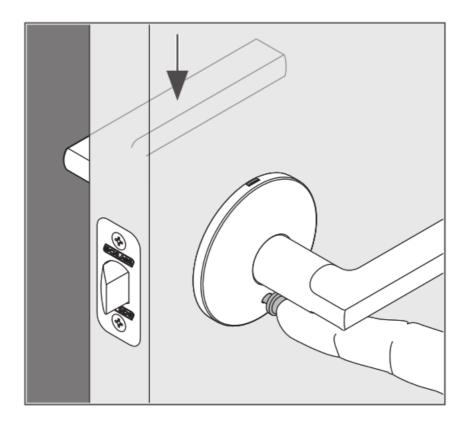
**7b** Use the emergency unlock tool to unlock the lock.
