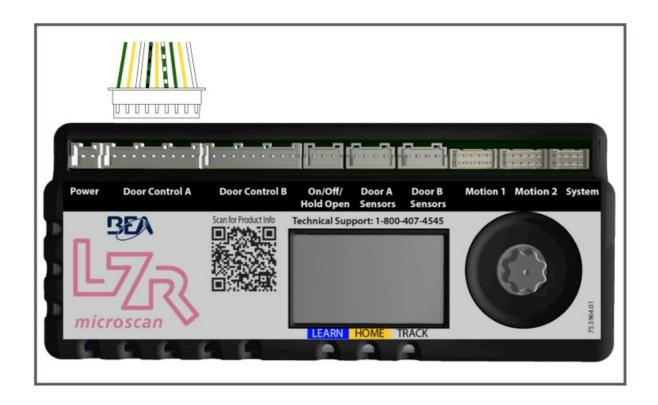
LZR-MICROSCAN T hub/sensors must be powered by a UL Class 2 power supply limited to 15 W. If a NEMA 5-15R outlet is not available in door header, cut off NEMA 5-15P plug and wire-nut to 110 VAC observing polarity and grounding.
