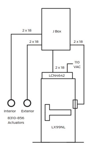
Operation: When the panic device is mechanically dogged both interior and exterior actuators will be enabled through LX switch. When device is undogged actuators will not function.
