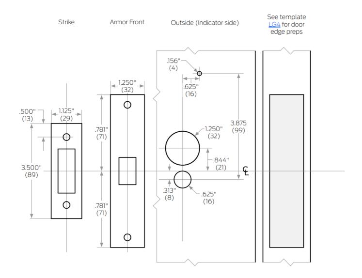
routing. Armor front deadbolt, auxiliary latch and latchbolt holes shown for dimensional purposes only. Use door edge measurements for door preparation.
