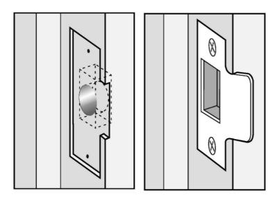
**NB** The plunger beside the latchbolt deadlocks the latchbolt and protects it against manipulation. IT MUST NOT enter the strike plate aperture when the door is closed.
