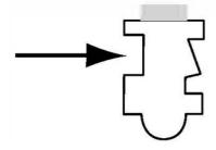
Section through lock case showing square notches in tumblers facing outwards
