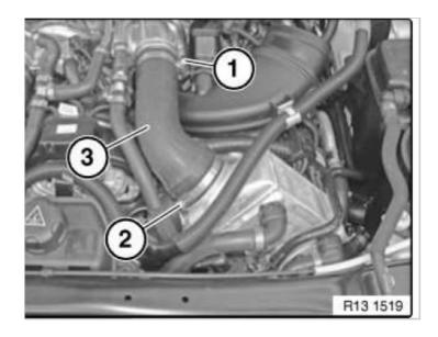
Release clamp (2). Replace clamp (2). Remove left charge-air duct (3).
