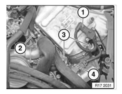
Unlock connector (1) and remove. Release screw (2). Tightening torque 13 71 6AZ.
