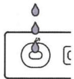
Secure white cap back on extraction tube and wait 15 minutes. 15 Min
