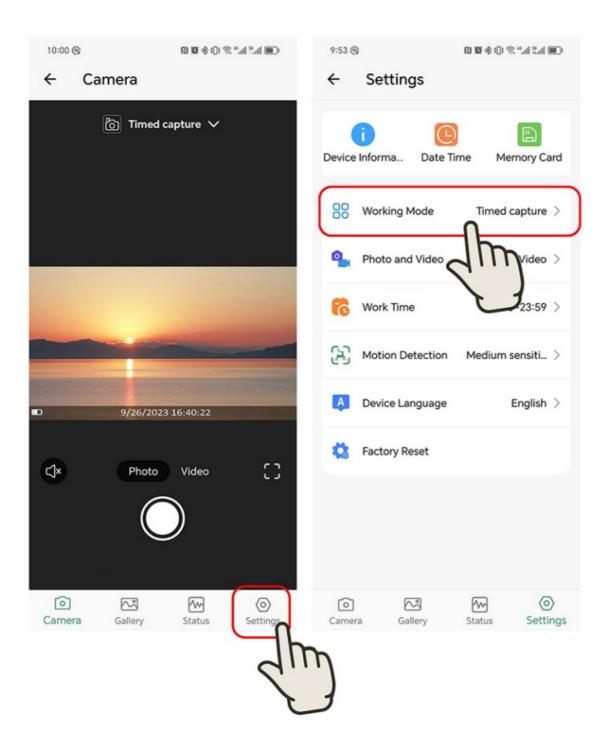
**Step 2:** Select "Timed Capture" from the "Mode" options. Choose the capture interval by specifying the desired time. Ensure to tap the "Confirm" button once all settings are configured.
