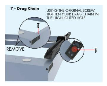
**STEP 4**Attaching Drag Chain to Y – Bracket
