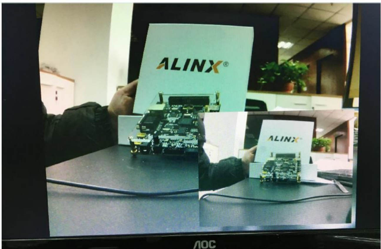
Figure 4-4: OV5642 Picture-in-picture Effect on the VGA Display
